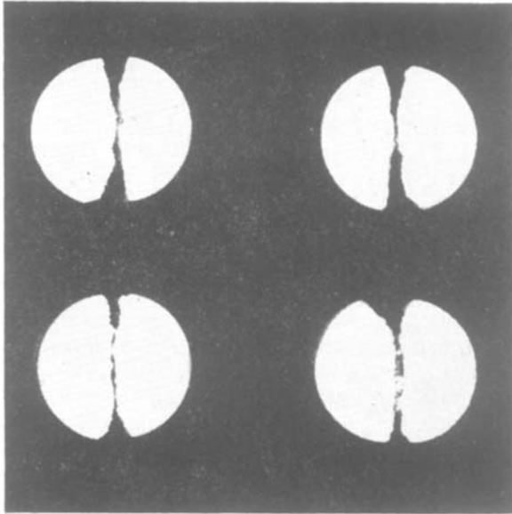
FIG. 5. Examples of the fracture of tablets. Upper row: Tablets made under high compression. Lower row: Tablets made under low compression. A similar wedge formation is shown by both series.
